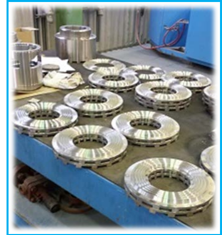
Figures 13 & 14 show internal locally manufactured components for isolation and control valves
